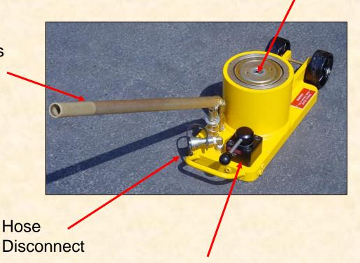
Shut-off Valve Allows Disconnect of Hose Under Load
