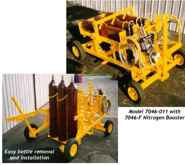
Our three bottle Nitrogen Servicing Cart is configured and designed for servicing aircraft tires, struts and accumulator systems. The low profile, low center of gravity and four-wheel design account for the trailer's stability and control during towing. The counter balanced 'tilt up-right" bottle rack makes loading and unloading bottles a one-person operation.
