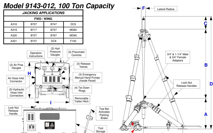
MODEL 9143-012 TRIPOD AIRCRAFT RECOVERY SYSTEM SPECIFICATIONS
