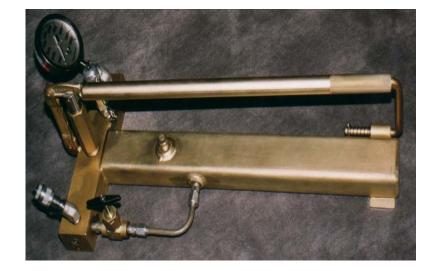
In Accordance with ANSI B40.1, the Model 7172-010, Pressure Gauge Calibration Unit, is a portable test unit which can be used to set and test U.S. manufactured gauges. This compact and lightweight unit can be easily carried around the hangar or to any remote jack location. The simple operation and simplistic design allows the operator to quickly calibrate gauges to airline calibration procedures while minimizing jack downtime.
